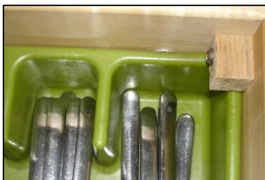
Flatware Tray Anchor (The anchor is shown in the front corner of the drawer. It keeps tray from sliding around the drawer.)
