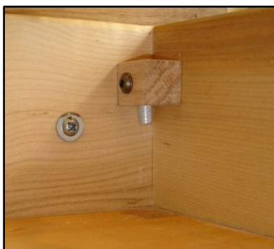
Anchor Block (The anchor is an aluminum rod in an oak block that is attached to the drawer with a screw. Lift other end of tray, to free tray from anchor.)
