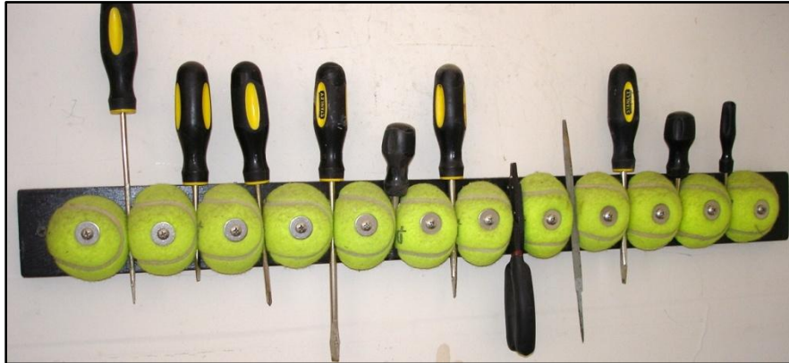
Tennis-Ball Tool Holder (The ½ ball shapes grip a range of tool sizes)
